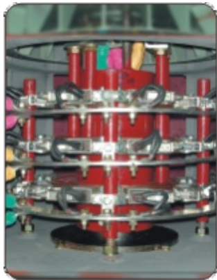
Fabricated Type Slip Ring Unit
